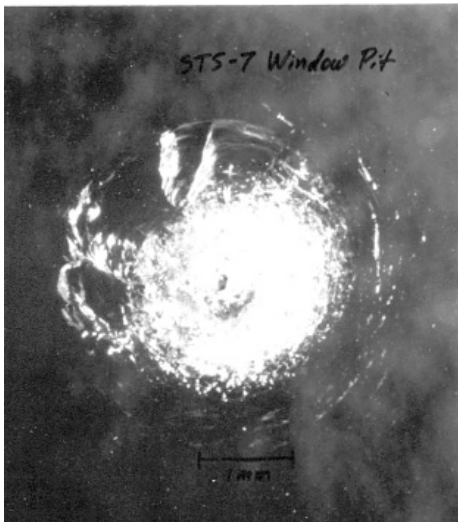
A fleck of paint left this crater on the surface of Space Shuttle Challenger's front window on STS-7.
